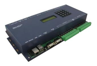
The EBox-AIO-001, which is designed for remote monitoring application of field device, meter or paired with SQL database to be a front-end controller to perform industrial tasks, such as data acquisition through TCP/IP, is based on the ATMEL ARM9 industrial processor, and features 8 digital input channels, and 8 relay output channels to do the switch control or status monitoring.
